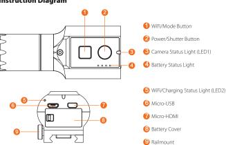
**Charging**Micro-USB supports DC 5-15V power supply. A DC 5V1~2A charger is recommended. The charging status light (red) will turn on during charging and turn off when charging is complete. It takes about 2 hours to get fully charged. **Battery Status**
