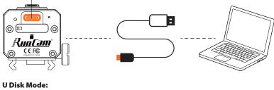
Connecting to PC via TYPE-C to USB, the camera will enter into U disk mode automatically, recording indicator(red light) is on WEBCAM/PCCAM/UVC Mode Short pressing WIFI button to switch to WEBCAM/PCCAM/UVC mode in U disk mode, then Short
