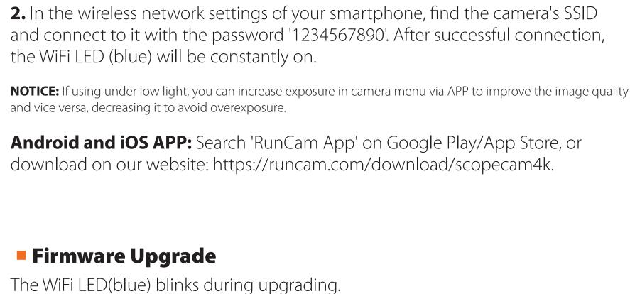
Manually copy the firmware file (RCSC4K.BRN) onto the microSD card. Follow the
